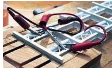
Figure 12: Floor, Step 4: clamping the bottom braces
