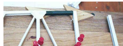
Figure 17: Side Truss, first top beam added
