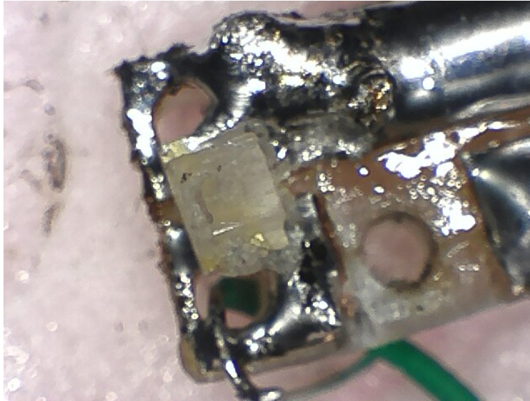
Figure 6.7 Signal Chip LED Soldered
