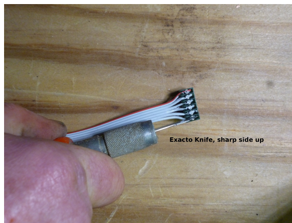
Figure 4.5 Installing Connector Plugs
