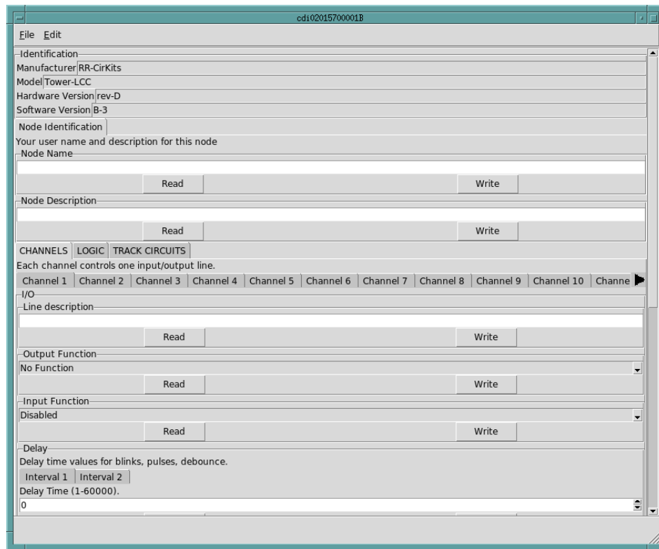
Figure 4.7 A CDI-based configuration screen for a RR-CirKits Tower-LLC node
